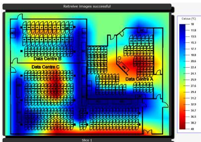
2. On-going real-time power, temperature and humidity monitoring with the results presented through an on-line dashboard on a 24/7 basis. The system allows users to set their own alarms, which automatically respond with text message alerts, and includes an audit trail of responses.
