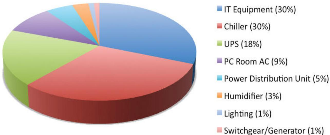
Of note, is that a significant portion of a datacentre's power consumption relates to cooling and humidity. It is for this reason that the **EDX DC-3** product has integrated granular level temperature and humidity elements into this offering to ensure that all of the environmental aspects of your data centre are in balance.
